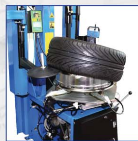
Mounting/removing device for low-profiled tires
