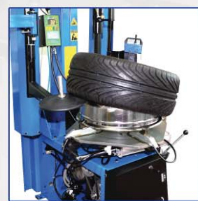
Mounting/removing device for low-profiled tires
