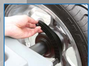
Automatic gauge arm : Automatic gauge of rim distance and diameter (Option for diameter)
