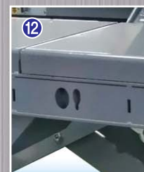
12 Alignment Cable duct Duct is provided for sensor connection of wheel alignment at the side of runway.
